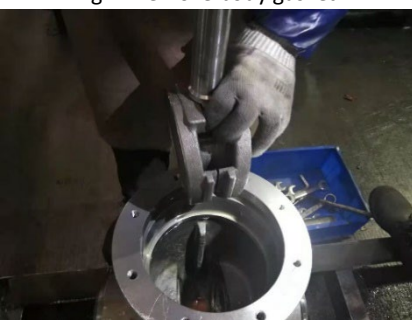
Fig.43 Lift up the wedge and disassembly stem & wedge
