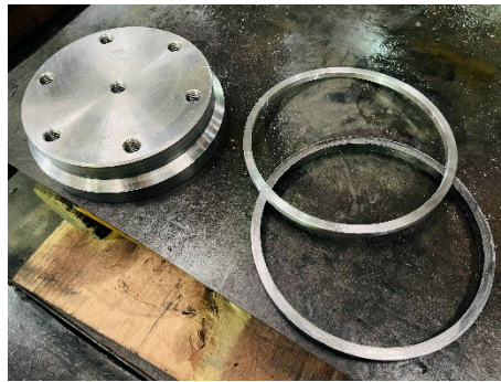
Fig.72 Remove pressure seal body gasket
